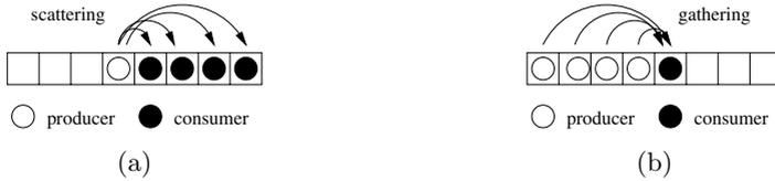
**Fig. 1.** Data access patterns. (a) Right-looking (scattering); (b) Left-looking (gathering).
